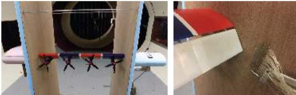
**Fig. 4 Photos of test rig. The left shows a front view of the setup, and the right shows a closeup of the wake survey rake.**
