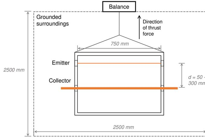
**Figure 2.** Schematic of thruster and thrust measurement setup. Side view of electrodes. Not to scale.
