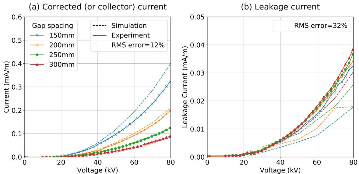
**Figure 9.** Experimental and numerical results for (a) corrected current (which is the current measured at the collector) and (b) leakage current. Results obtained by matching the boundary conditions and electrode potentials in simulations to those in experiment.
