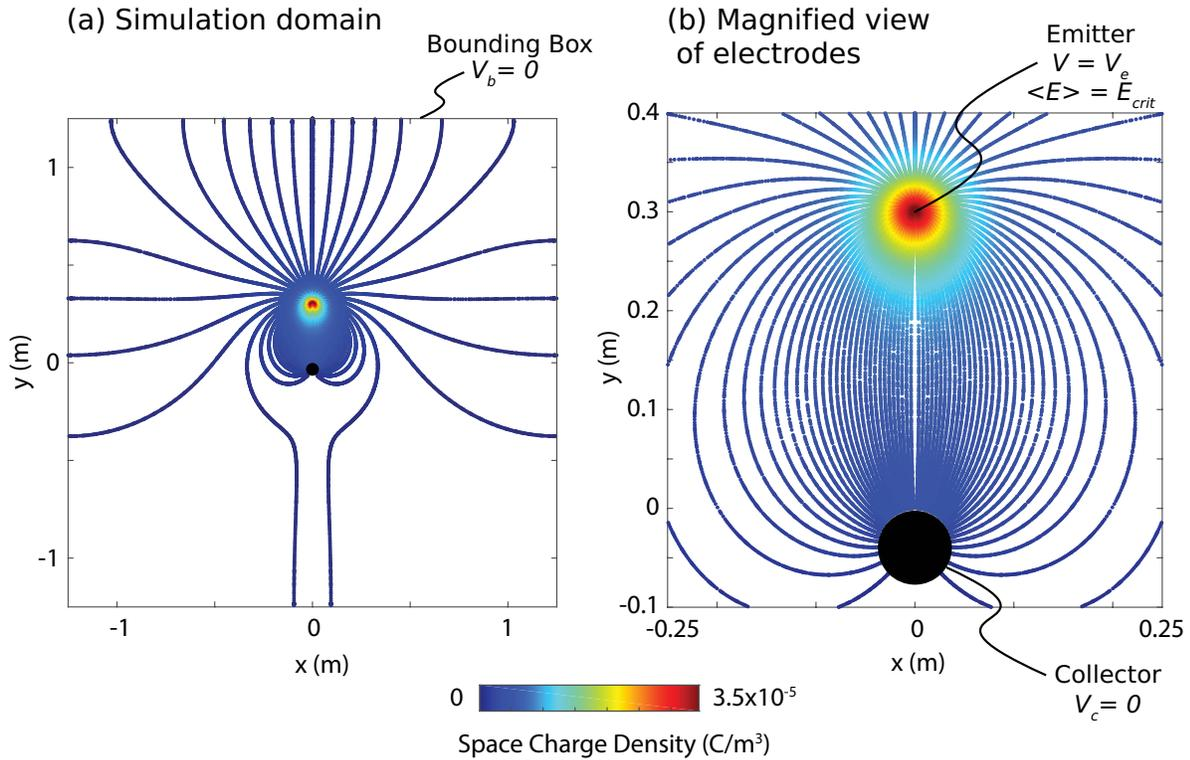
**Figure 8.** (a) Entire simulation domain and (b) magnified view of electrodes, showing current paths. Large black circle is the collector. Boundary conditions are indicated. Simulation conditions:  $V_e=80$  kV,  $V_c=0$  kV,  $V_b=0$  kV,  $d=300$  mm,  $2r_c=38$  mm.
