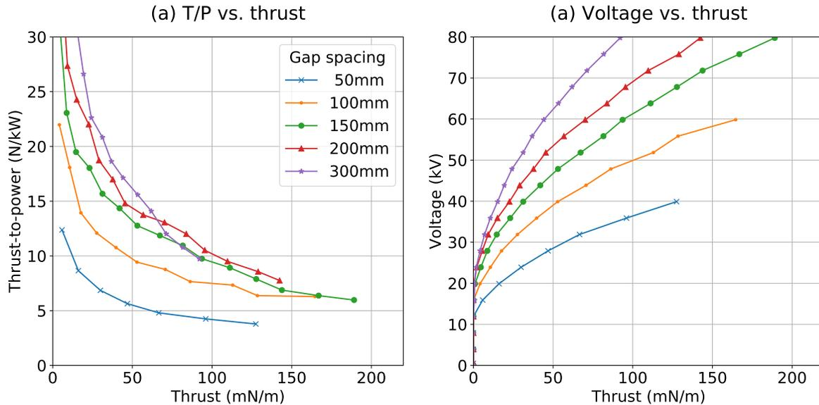
**Figure 7.** (a) Thrust-to-power versus thrust, and (b) voltage versus thrust for different gap spacings using a differential  $V_e = 0.5V_a$  power supply configuration and a 38 mm collector. Power is calculated using the total drawn current, which is the maximum current recorded at either electrode. In differential mode, the net leakage current is approximately zero, and the measured difference between the emitter and collector currents is less than 2% in all cases.
