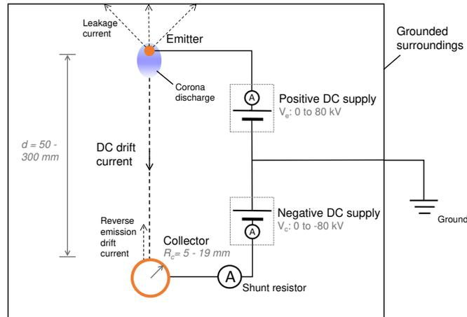
**Figure 1.** Electrical schematic of experimental setup. End view of electrodes. Some experiments used the positive DC supply only. Power supplies have internal current and voltage measurement. An independent shunt resistor is used to measure current through the collector when the negative DC supply is not used. Not to scale.
