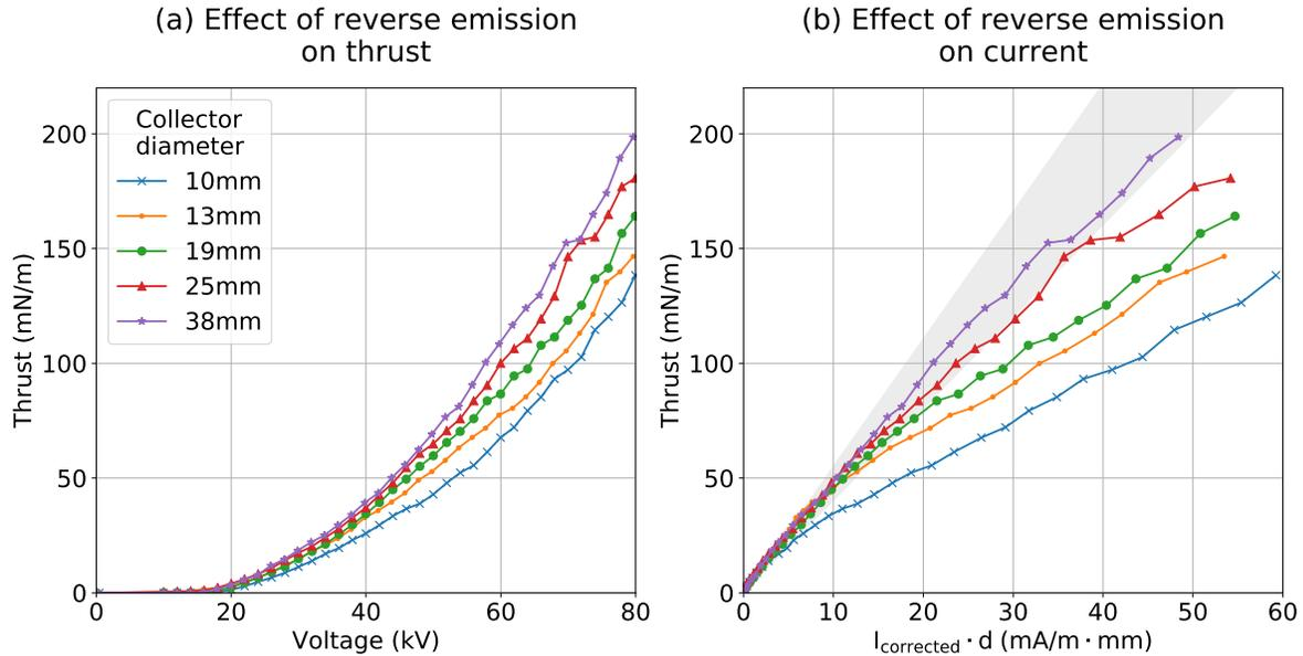
**Figure 5.** (a) Thrust vs. voltage (b) thrust vs. the product of current and gap spacing at 150 mm gap spacing for varying collector diameters. Lower thrust and higher current draw for smaller collector diameters is consistent with reverse corona emission at the collector electrode.
