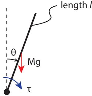
Figure 3.2: Definition of parameters for rigid pendulum.
