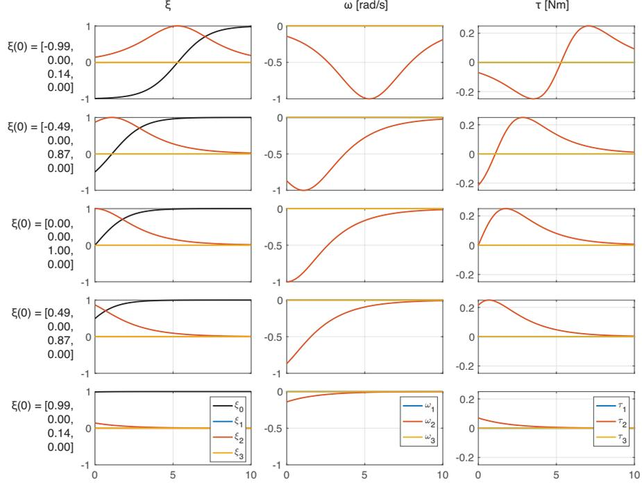
Figure 3.1: Analytic Controller. Each row represents the solution from a different starting quaternion, indicated on the left. The columns show the quaternion components, the angular velocity and the torque applied.
